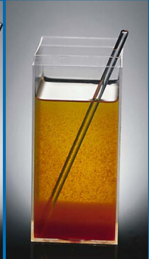
Sol undergoes coagulation upon the addition of Al 2 (SO 4 ) 3 solution
