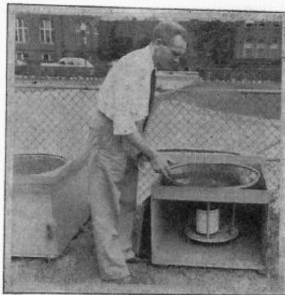
FIG. 1—Evaporimeters at Urbana, Illinois, evaporation station
